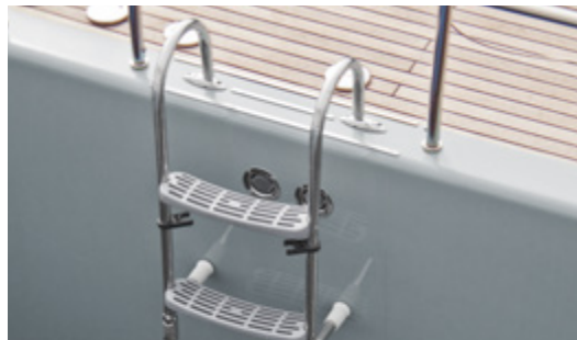
Stainless steel removable ladder to rail gate exit
