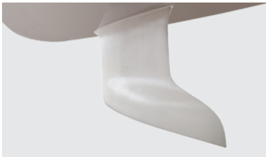
Shallow draft L-shape keel (1.82 m), cast iron
