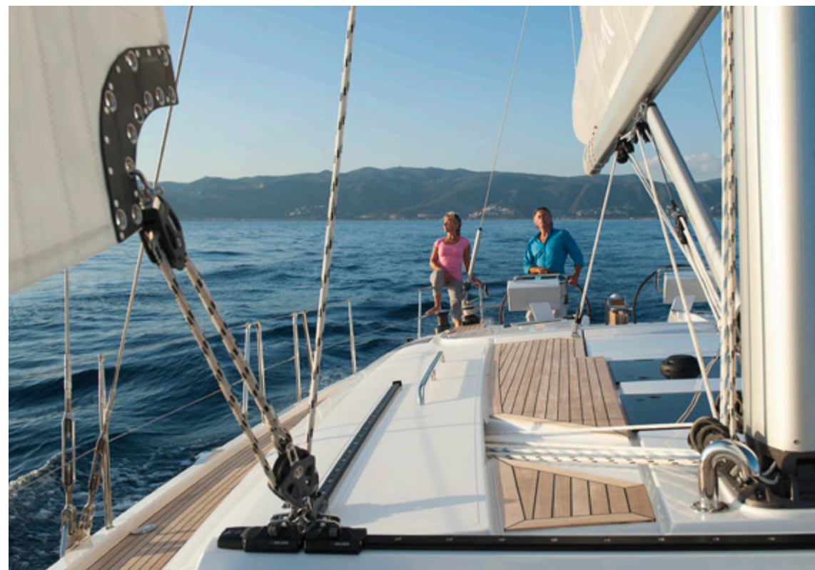
3 Integrated self-tacking jib track with „high-load“ slide system.
