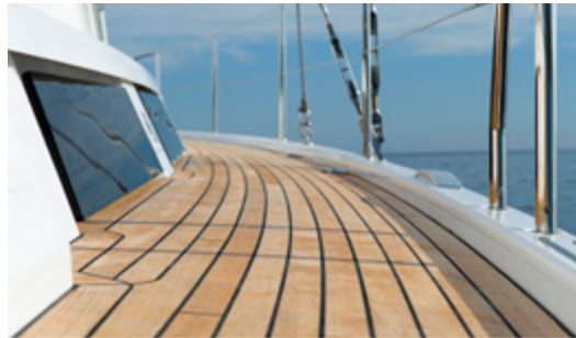
Classic teak decking on side decks and coach roof
