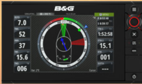
2 B&G Zeus² 9 chart plotter, one at each helm position, 2 Navpods, one per steering pedestal
