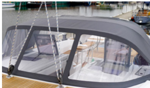
Sprayhood with stainless steel frame and large windows
