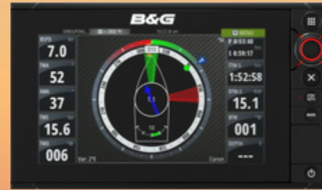
2 B&G Zeus² 9 chart plotter, one at each helm position, 2 Navpods, one per steering pedestal
