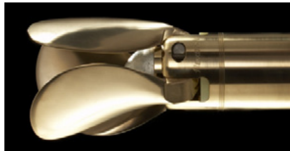
Three blade folding propeller, Volvo D2-75
