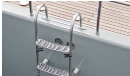
Stainless steel removable ladder at guard rail exit
