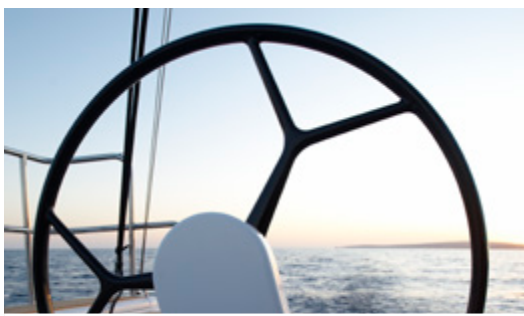
2 Steering wheels, Y-spoke-design, GRP-composite, black or white colour
