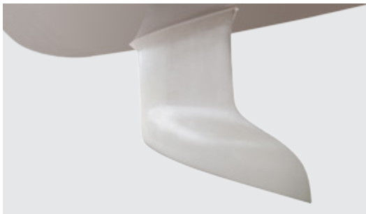
Shallow draft L-shape keel (1.98 m), cast iron
