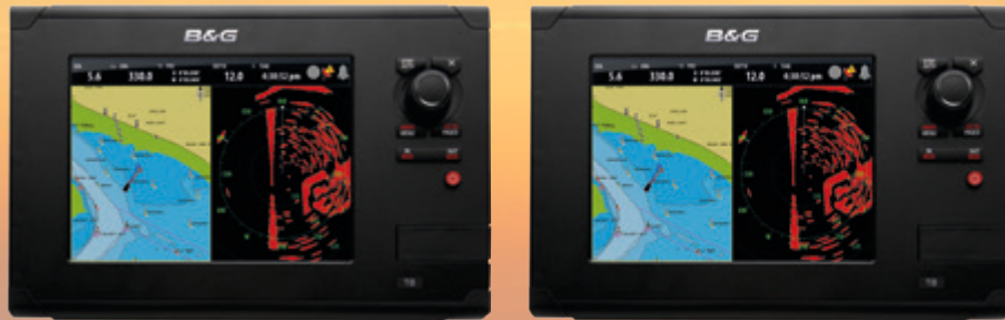
2 B&G Zeus touch 8 GPS chart plotter, one at each helm position
