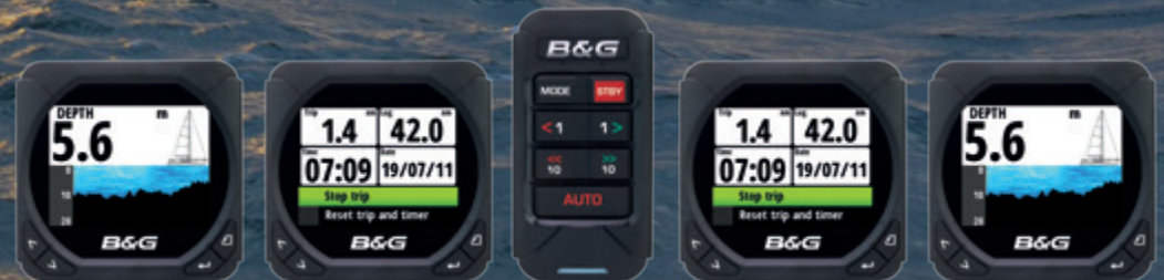
4 B&G Triton multifunction displays, two at each helm position, incl. windtransducer, Autopilot B&G control unit & FluxGate Gyro Compass RC42, AIS Class B transponder, NMEA engine information interface for chart plotter, Antenna splitter for VHF and AIS
