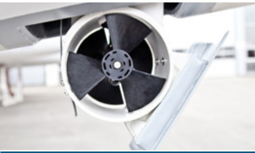
Retractable bow and sternthruster
