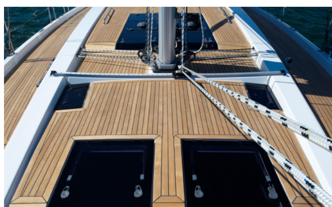
3 Self-tacking jib system with integrated track. Tacking with no need for grinding.
