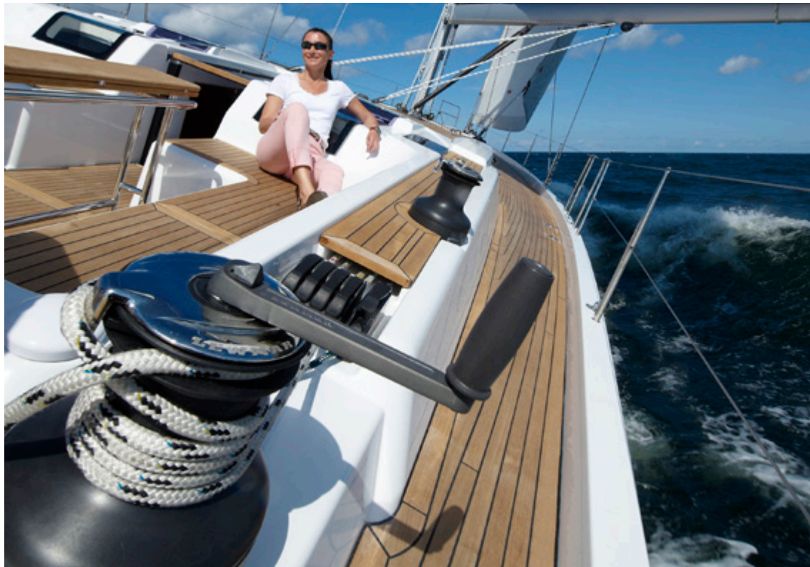
3 Easy sailing: Halyards, sheets and reef lines running to helmsman position.
