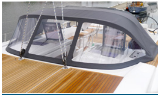
Sprayhood with stainless steel frame and windows
