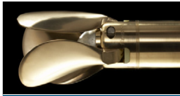
Three blade folding propeller, Volvo D3-110/150
