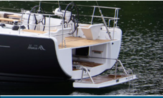
Easy tender system with hydraulic platform
