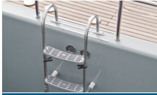
Stainless steel removable ladder at rail gate exit
