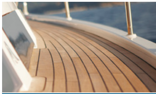
Classic teak decking on side decks and coach roof
