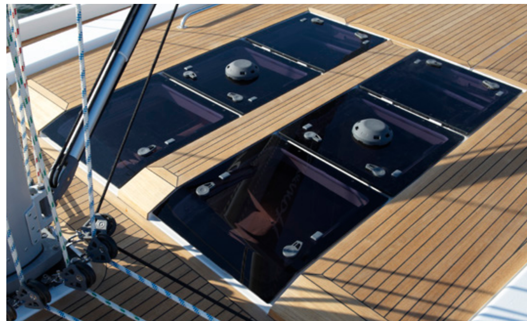
3 Elegantly designed and openable flush hatches above the saloon for light and ventilation.
